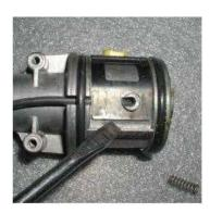
4. REMOVE PHILLIPS SCREW FROM #27 SOCKET WITH SMALL JEWELERS SCREWDRIVER. YOU CAN THEN REMOVE THE IGNITER WIRE.
