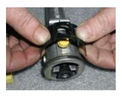
7. REMOVE THE #7 RETAINER FROM THE #8 INLET AND THE UNDERLYING #6 O-RING. REMOVE THE FILTER HOLDER. CLEAN THE FILTER SCREEN AND REPLACE. REPLACE THE #2 O-RING AND REASSEMBLE. INSERT #6 O-RING AND RETAINER.
